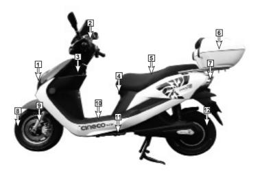
1. Headlamp 2. Instrument 3. Document box 4. Charging interface 5. Seat 6. Trunk 7. Tail lamp 8. Front wheel 9. Front shock absorber 10. Front pedal 11. Side stand 12. Rear wheel
