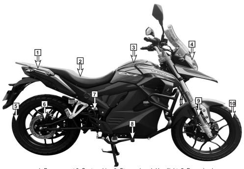
1. Rear armrest 2. Seat cushion  $\overline{3}$ . Storage box 4. Headlight 5. Rear wheel 6. Rear disc brake 7. Motor 8. Rear brake pedal 9. Front shock absorber 10. Front wheel
