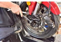
Loosen (but do not remove) the Allen pinch bolts at the bottom of the fork legs (there are two on each fork).
