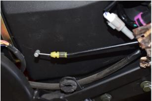
There is no adjustment for the rear seat release cable. The throttle cable should be adjusted such that there is 2 to 5 degrees of free rotation before the throttle is actuated. This accomplished through use of the adjustment mechanism underneath the right handlebar.
