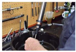
Inspect the condition of the seals, the spring, the fork lower plated surfaces, and the bushings. If any parts are damaged, please contact CSC for replacements at 909 445 0900.
