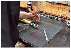
After unscrewing the fork cap assembly, remove the fork spring.
