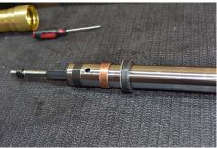
The fork capacity is 270cc in each fork leg. We generally use 10W fork oil when replacing the fork oil. Please contact CSC at 909 445 0900 if you need fork oil.
