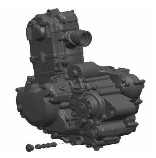
This is what the strainer and filter caps look like on the engine. The oil strainer is the large 17mm bolt head, and the oil filter cover is held in place by two 8mm nut on the right, and the left oil strainer is
