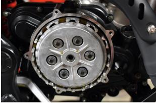
Set the clutch cover aside, inside face up, so that you can use it as container for the parts to be removed next. Remove the six clutch pressure plate bolts. Each bolt has a machined keeper and a spring.
