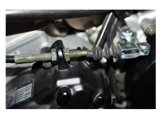
Once you've done adjusted the lower end of the clutch cable, adjust the knurled adjustment know at the handlebar clutch lever such that there is about 10mm to 20mm of free play at the end of the clutch lever. When you've done that, lock the knurled adjustment knob in place with the knurled lock nut. Pull the rubber grommet back over the adjustment mechanism.
