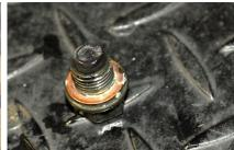
The oil drain plug has a copper gasket. It is not necessary to replace this unless oil leaks from around the drain plug. The drain plug has a magnetic core. Wipe it clean.
