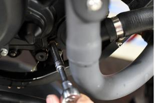
Allow the cooling fluid to completely drain from the radiator. Move the bike to a completely vertical orientation to allow the radiator to drain completely.
