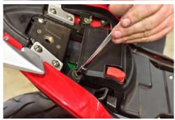
After removing the seats, remove the cover over the battery.
