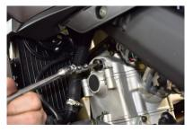
The next step is to pull the wire off of the spark plug and then remove the spark plug.
