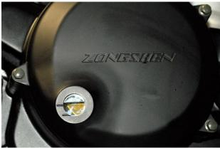
Reinstall both oil fill caps (the one with the slot and the one with the extension for turning by hand). Start the motorcycle and let it run for a couple of minutes, and check for leaks.
