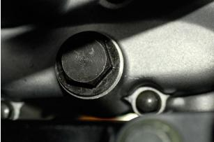
Use a 17mm socket with an extension to remove the oil strainer caps. Use an 8mm socket and an extension to remove the oil filter cover. We can provide these tools to you as part of an oil change service pack; we also sell the oil change tool kit separately if you do not have these tools.
