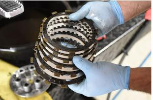
If the clutch slips due to the use of an unapproved oil (for example, an automotive oil with friction inhibitors), wash the plates to remove any remnants of the unapproved oil that induced the slippage.
