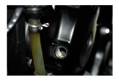
Next, remove the view caps on the left cylinder head. They can be removed with a 6mm Allen wrench. These view ports will allow determining that the engine is at top dead center.
