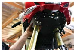
Using a small screwdriver, gently pry the lower fork seal away from the fork upper. Caution! Take care not to scratch or gouge the fork upper.
