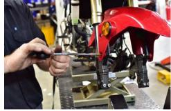
Loosen (but do not remove) the two Allen pinch bolts on the upper triple tee.
