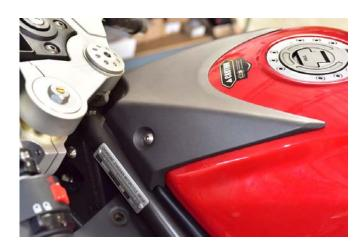
The fuel tank forward panel is retained by two bolts.
