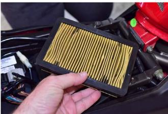
After repeated cleanings, or when the air filter element ages, it will ultimately need to be replaced. If you need replacement air filter elements, call CSC for a replacement element.
