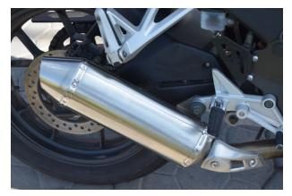
The exhaust system functions are to discharge exhaust gas, to reduce noise, to eliminate flames or sparks from the exhaust, and to assist in the emissions control process.
