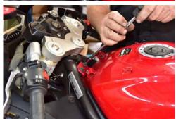
Lift the fuel tank by rotating it at its rear hinge. It is best to do this with little fuel in the fuel tank. This will provide access to the fuel pump.
