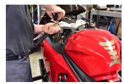
Remove all of the fasteners securing the side and lower body panels.
