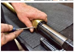
Fully unscrew the damping adjuster until it can no longer be turned.
