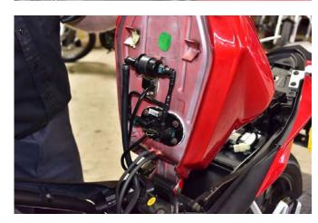
After removing the two forward fuel tank retaining bolts, you can tilt the fuel tank rearward to provide access to the fuel system components.
