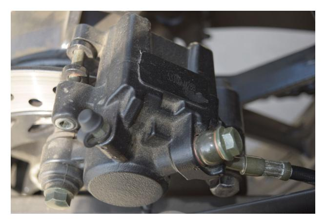
Once the caliper bolts are removed, the pads will slide out. Inspect the brake pads to determine if they are worn beyond their service limit (less than 1.5mm thick). If the pads are worn such that the grooves are gone (visible as vertical slots in the photo above), the pads should be replaced.
