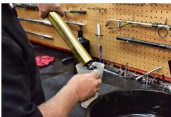
Next unscrew the fork cap assembly from the fork internal rod. This is made challenging by the fork spring and the lock nut arrangement securing the fork internal rod to the fork cap assembly.
