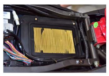
Remove the air filter for cleaning or replacement.
