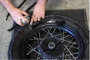
Using a tire iron (you'll need two), insert the tip between the tire and the bead, and pull the bead over the rim. Using the second tire iron, pick a location about 6 inches away (measured circumferentially on the rim) and do the same thing. Remove the first tire iron and repeat the process. Remove the tire from the wheel.
