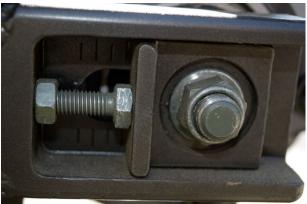
Move the rear axle either forward or rearward using the rear axle adjustor nuts while simultaneously positioning the rear axle such that the desired chain tension is achieved and the rear wheel is aligned.
