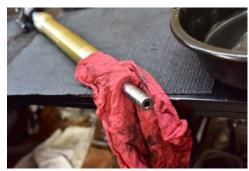
The fork contains oil, and when you remove the cap assembly, tilting the fork down will allow the oil to drain. Drain the oil into a receptacle.
