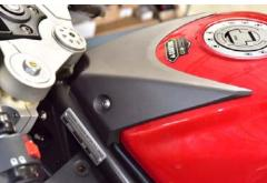
Unbolt the fuel tank at its forward edge.
