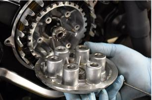
There's a pusher behind the pressure plate that consists of a shaft, a roller bearing, and washer. You can see it in the photo above, and here are additional photos that show these components.
