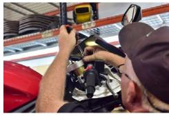
While holding the fork, loosen (but do not remove) the lower triple tee Allen pinch bolts. Caution! When both are loose, the fork will be free to fall, so make sure you are holding it as these bolts are loosened.
