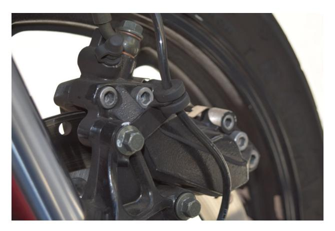
Remove the caliper and then remove the bolts from the caliper. Inspect the front brake pads and replace if necessary. Reinstall the caliper bolts and the caliper. Tighten all fasteners. Pump the front brake lever several times. Operate the motorcycle to assure satisfactory front brake performance.
