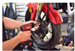
Loosen (but do not remove yet) the front axle bolt.
