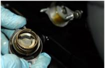
Once you have removed the filter cover, you'll see the metal end of the oil filter, as shown in the photos below. Slide the oil filter out of the engine. The easiest way to do this is to take the magnetic drain plug, put the magnet end against the oil filter, and slide it out. The oil filter end with the rubber gasket goes into the engine first. Install a new oil filter with each oil change.
