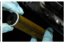
Next remove and clean the oil strainers. Remember that there are two (one on each side of the engine). You can pull the oil strainers out of the engine using a pair of needle nose pliers. You can clean the oil strainer using WD40 or compressed air.
