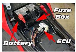
To get to other electrical system components, it is necessary to rotate the fuel tank to the rear. Remove the fuel tank upper body panel.
