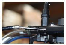
Once you have enough slack in the clutch cable, you can remove the cable sheath from the knurled adjustment knob at the handlebar end of the cable, and slide the clutch cable out. This will allow pulling the cable forward and sliding the cable head out of the clutch lever (as shown to the right).
