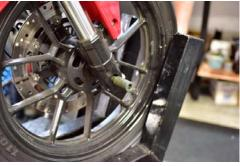
Note that there are two bushings (one of each side of the front wheel) between the front wheel and each front fork.
