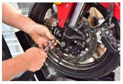
Remove the front axle nut on the left side of the motorcycle and pull the axle out to the right.
