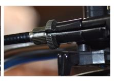
Locate the other end of the clutch cable where it attaches to the clutch lever on the engine case. It's on the left side of the engine behind the cylinder and above the shift lever. Loosen the lock nuts on the threaded adjustment mechanism and move it forward to gain more slack in the cable.
