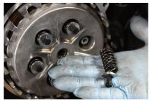
Remove the clutch pressure plate. You may need to use a small pick to get behind it to coax it out.
