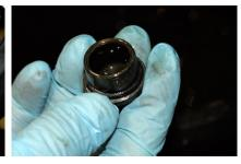
Next, remove the oil filter cover. It is secured by two 8mm nuts. You can attempt to remove these with the 8mm wrench provided with the RC3 tool kit; a much better approach, though, is to use an 8mm socket with an extension. Remove the two 8mm nuts and the access port and set them aside, taking care not to lose the nuts. The oil filter cover also has an O-ring. Take care not to get the O-ring dirty or lose it. The spring inside the cover is orientation insensitive; it can be inserted either way.
