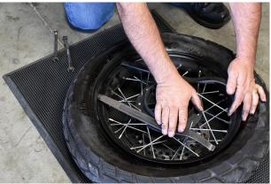
Install the new tire on the rim using tire irons. Inflate the tire until it seats on the wheel rim. Liberal use of spray lubricant will help to seat the tire bead on the rim. Once the tire bead is seated on both sides of the wheel rim, deflate the tire.
