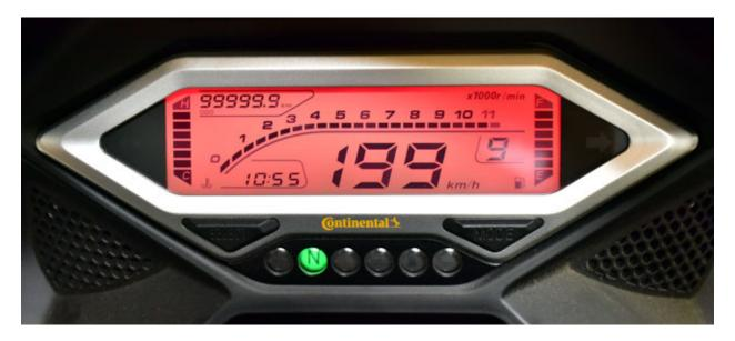
Other than replacing the indicator light bulbs, the instruments are not designed to be repairable. If any of the instruments fails, the instrument cluster must be replaced.
