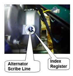
Align the scribe line with the index register in the center of the viewing port on the engine crankcase and the "L" and "R" marks are visible in the cylinder head viewing ports. There are scribe lines on the cam chain sprocket next to the "L" and "R" marks, these should be aligned with the machined marks in the viewing ports' threaded regions as shown below. When these marks are aligned (as shown below), the scribe line will be visible in the crankcase viewing port.
