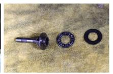
Inspect the roller bearing and washer. If either part is damaged, replace it.
