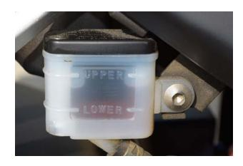
Using a turkey baster or other suction device, remove as much of the brake fluid in the master cylinder as possible. **Caution!** Exercise caution to prevent any brake fluid spillage. If any spillage occurs, wipe up the spilled brake fluid immediately (it will damage painted or plastic surfaces). Remove the caliper bleed cap and attach a small diameter tube to the caliper bleed fitting. Route the tube to a receptacle. (Note: The photos shown here are for the RX3; the RC3 is similar.)
