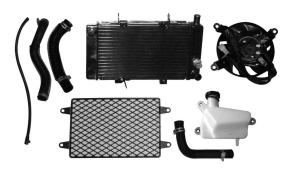
Radiator: The radiator is exposed in the air and located on the windward side of the motorcycle, where the high-temperature water dissipates the heat from the engine into the air and becomes low-temperature water.
