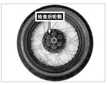
[12] Check whether the rear wheel bearing is worn. When the rear wheel bearing is worn, the rear wheel bearing shall be removed for replacement.
