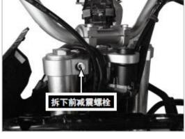
Remove the front shock absorbing bolt
