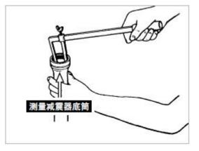
Measuring shock absorber bottom cylinder
