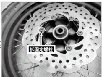
Remove the fixing bolt
