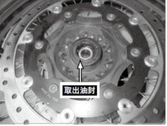
[6] Place the front wheel on the calibration table, rotate the front wheel at high speed by hand, and check the wear and free travel of the front wheel axle. Check whether the front wheel bearing is worn. When the front wheel bearing is worn, the front wheel bearing needs to be removed for replacement.
