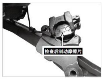
Check rear brake friction plate
