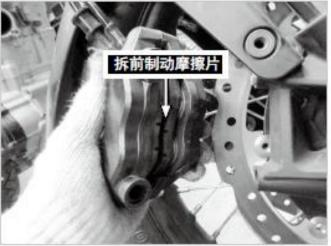
Remove the front brake friction plate
