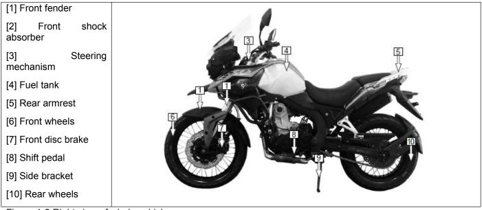
Figure 1-2 Right view of whole vehicle
