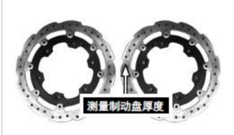
Measuring brake disc thickness
