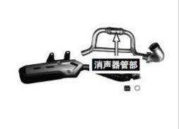
Muffler pipe section
