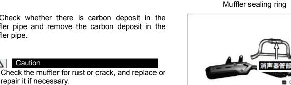
[5] Check whether there is the carbon deposit in the tail of the muffler and remove the carbon deposit in
