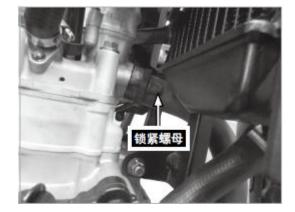
[2] Remove the muffler. Check whether the silencer is broken or damaged. When the silencer is broken or damaged, the silencer shall be welded or replaced.
