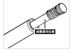
[2] Check whether the spring lengths of the left and right rear shock absorbers are consistent, check whether there is crack or damage on the spring surface of the shock absorber, and replace the rear shock absorber if necessary.
