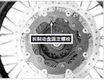
Remove the brake disc retaining bolt
