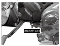
[1]Dismantle the fixed bolt of gearshift pedal and remove the gearshift pedal.
