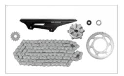
The rear transmission device of this motorcycle adopts chain. It mainly consists of drive gear, driven gear, drive chain, chain tie-in, drive chain box, chain adjuster and rubber dead block.
