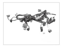
[6]Check whether the main cable is damaged. Bundle the leads in time if the insulative rubberized fabric is damaged.
