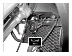
[5]When the sound of electric horn is hoarse and electric horn has no sound, adjust the horn volume according to the actual situation or replace the horn with the same type.
