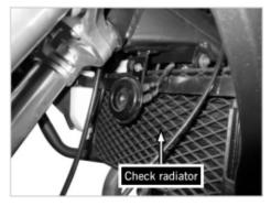
[2]Check the abrasion of radiation pieces of radiator and whether they have water leakage.
