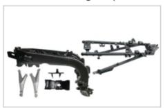
The frame of this motorcycle adopts pipe jointing and crooked girder. It has high intensity,good firmness and good suitability. It mainly consists of head pipe, main frame, tail pipe,rear supporting pipe and low bending pipe. It is made through the methods of jointing, riveting and so on.
