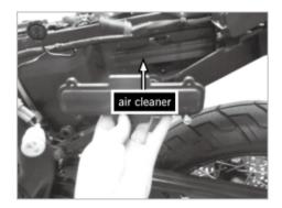
[2]Dismantle lock screw of air cleaner element. Take out the element of air cleaner and check whether there is too much dust on it. Clean it if too much dust.
