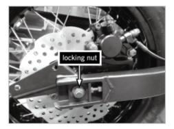
[11]Disassemble the nut of rear wheel axle and remove the wheel axle and rear wheel assembly.
