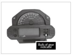
[4]Check whether the bulb of meter indicator is burned-out. Replace it if burned-out.
