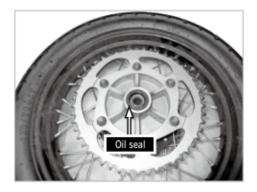
[7]Remove the oil seal of cushion body of rear drive sprocket wheel and check its abrasion.
