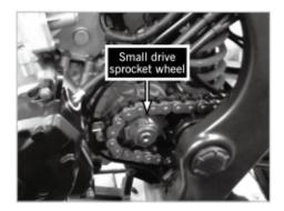
[4]Dismantle fixed bolt of chain box, and remove the chain box.
