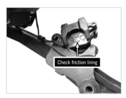
[12]Remove friction lining and Measure the thickness of it with the limit value of repair is 2.0mm.
