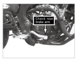
[10] If the free stroke of rear brake pedal cannot reach the standard value, readjust the nut of rear brake rod.
