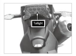
[4]Check whether the taillight is burned-out. Replace it with the same type if burned-out.
