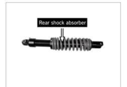
[2]Check whether the left one has the same length as the right one and check whether the spring surface of shock absorber is damaged. Replace it if damaged.
