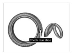
[17]Check the rear shoe for wear. The limit value of repair for tread of rear shoe is 2.00mm.
