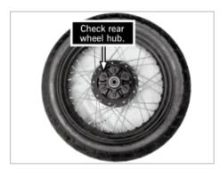
[12]Check whether rear axle is worn.Replace it if worn.
