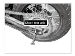
[11]Dismantle rear wheel and check whether rear wheel hub is damaged. Replace it if damaged
