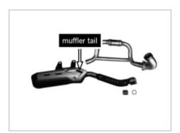
[5]Check whether there is carbon deposit at the muffler tail.Clean it.
