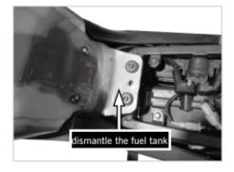
[5]First of all, dismantle the left and right side cover and seat. Then remove fixed bolt and take out the fuel tank.
