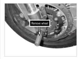
[4]Disassemble locking nut of front axle and Mileage line, then remove the front wheel.
