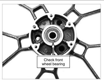
[6] Place the front wheel on the calibration table, rotate the front wheel at high speed by hand, and check the wear and free travel of the front wheel axle. Check whether the front wheel bearing is worn. When the front wheel bearing is worn, the front wheel bearing needs to be removed for replacement.
