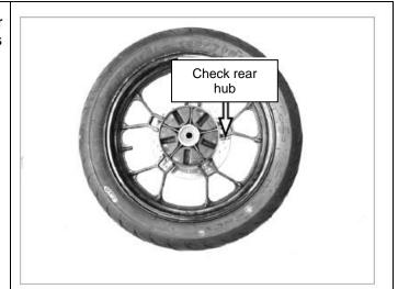
[12] Check whether the rear wheel bearing is worn. When the rear wheel bearing is worn, the rear wheel bearing shall be removed for replacement.
