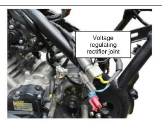
[1] Use a multi meter to measure whether the output voltage of the voltage regulating rectifier is within the range of  $13.0V \sim 14.0 \text{ V}$ . When the output voltage of the voltage regulating rectifier is lower than 13.0 V, the voltage regulating rectifier needs to be replaced.
