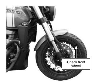
[3] Before removing the front wheel, the motorcycle body must be fixed firmly to keep the front wheel off the ground, then remove the front wheel axle fastening nut, take out the front wheel axle, and take down the front wheel assembly.
