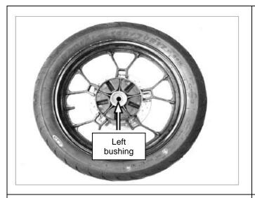
[7] Remove the rear axle lock nut and the rear wheel assembly. Remove the rear wheel left bushing and check the rear sprocket left bushing for wear.
