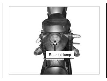
[2] Check whether the tail light is burnt out. When the tail lamp is burnt out, replace the same type of tail light.
