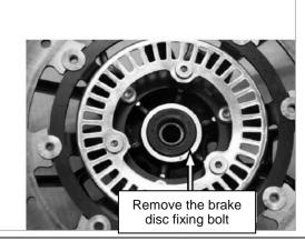
[6] Remove the front wheel, remove the front brake disc fixing bolt, and take out the front brake disc.
