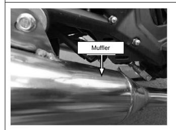
[2] Remove the muffler. Check whether the silencer is broken or damaged. When the silencer is broken or damaged, the silencer shall be welded or replaced.
