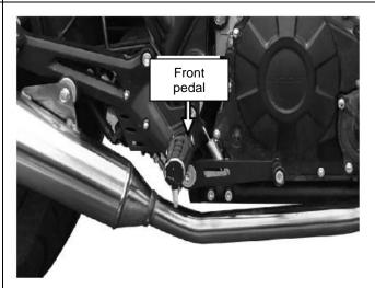
[6] Check whether there is looseness at the engagement between the shift pedal and the shift shaft, and also check whether the threads of the shift pedal adjusting rod are damaged.
