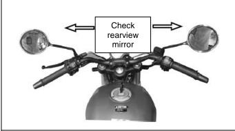
[1] Check whether the rearview mirror is loose or damaged. If the rearview mirror is loose or damaged, fix and replace the rearview mirror in time.
