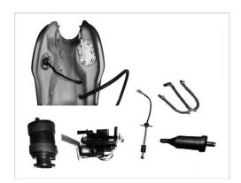
The fuel filter is connected in series on the oil path between the electric fuel pump and the fuel rail. In order to ensure the filtering effect and prevent the nozzle from clogging due to foreign matters, the system needs to adopt a special fuel filter for EFI. The shell of the filter must be strong enough not to be cracked due to fuel pressure.
