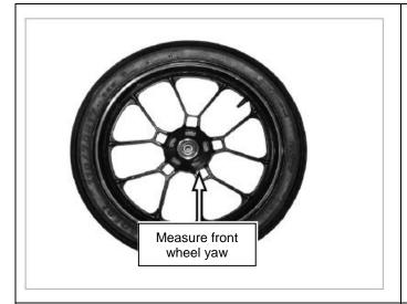
[8] Place the front wheel on the calibration table, check the deflection of the front wheel, rotate the front wheel by hand, measure the deflection value of the front wheel with a dial indicator, and read the deflection value shown.
