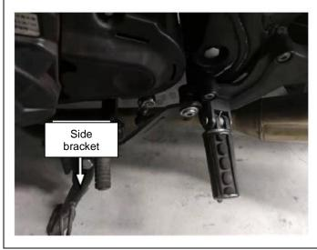
[2] Check whether the side bracket is bent or deformed, and replace or correct it when the side bracket is bent or deformed.
