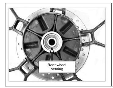
[10] Remove the inner bushing of the rear drive chain wheel and check the wear of the rear drive chain wheel bearing. When the bearing is worn, it should be replaced in time, otherwise it will affect the normal operation of the transmission system.
