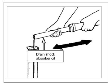
[3] Remove the front shock absorber drain bolt. Pour out the front shock absorber oil and check whether the front shock absorber oil is deteriorated. When the front shock absorber oil is deteriorated, replace the front shock absorber oil.
