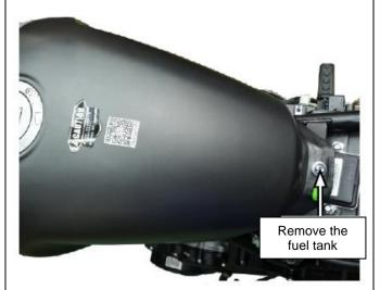
[5] First remove the left and right side covers and seat cushion. Then remove the fuel tank fixing bolt and take out the fuel tank.
