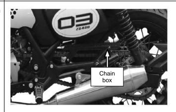
[6] Check the wear and deformation of the transmission chain, and replace the large and small transmission chain wheels and the transmission chain in a complete set according to the actual wear of the transmission chain.
