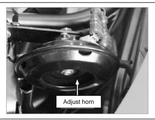
[5] When the sound of the electric horn is hoarse and the electric horn has no sound, adjust the volume of the electric horn according to the actual situation, or replace the electric horn of the same model.
