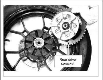
[9] Take out the rear drive sprocket and check the wear condition of the rear drive sprocket.
