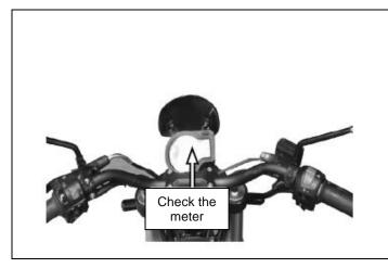
[1] When each indicator of the meter cannot work normally, the mileage meter shall be removed for inspection.
