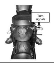
[3] Check whether the steering lamp is burnt out. If it is burnt out, replace the steering lamp of the same model.
