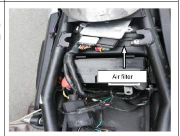
[2] Check whether there is too much dust in the filter element of the air cleaner. If there is too much dust in the filter element, replace the filter element.
