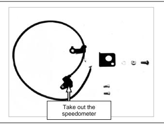
[5] Take out the speedometer and check whether the oil seal edge of the speedometer is worn or damaged. If the oil seal edge of the speedometer is worn or damaged, it should be replaced.
