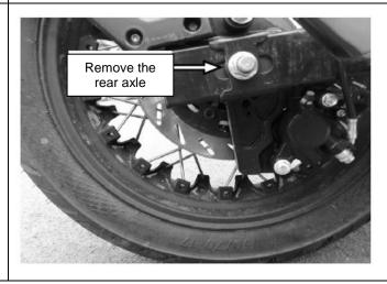
[11] Remove the rear wheel, check the rear hub for damage, and replace it when the rear wheel hub is damaged.
