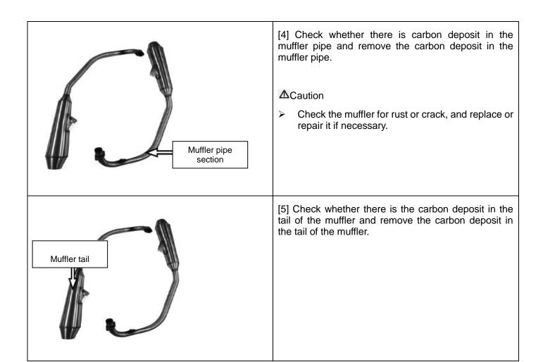
V. Intake and Exhaust System Damage Forms, Fault Phenomenon and Common Maintenance Methods are Shown in Table 3-3:
