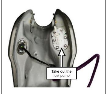
[7] Remove the fuel pump. Clean the oil residue and water in the fuel tank with cleaning agent.
