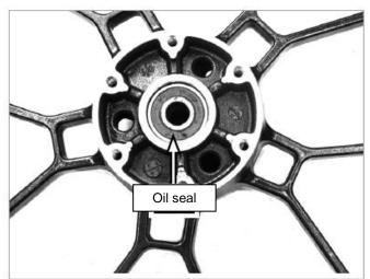
[8] Remove the rear drive sprocket oil seal and check whether the rear drive sprocket oil seal is worn.
