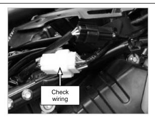
[3] Check whether the instrument wiring is loose.
