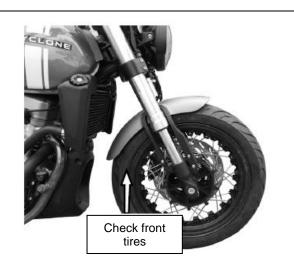
[1] Check whether the tire pressure is kept within the normal pressure range, remove foreign matters in the tread pattern of the outer tire, maintain the adhesion between the tire and the ground, and prevent sharp objects from damaging the inner and outer tires.
