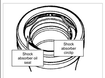
[4] Remove the front shock absorber oil seal and clamp spring, check whether the cutting edge of the front shock absorber oil seal is worn, and replace the front shock absorber oil seal.
