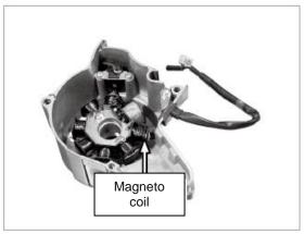
[4] Remove the engine left box cover, take out the magneto stator, and use a universal meter to measure whether the magneto stator resistance is short-circuited or open-circuited. If the magneto stator resistance is short-circuited or open-circuited, replace the magneto stator.
