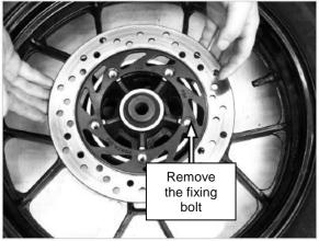
[13] Remove the rear brake disc fixing bolt and take out the rear brake disc.
