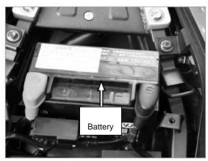
[2] Take out the storage battery and use a multi meter to measure whether the voltage at both ends of the storage battery is above "12V". When the voltage of the storage battery is below "12V", the storage battery needs to be taken off for charging.
