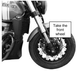
[4] Remove the fastening nut of the front axle, the soft axle of the mileage line and the front wheel.
