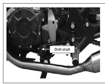
[1] Remove the retaining bolt of the shift pedal and remove the shift pedal.
