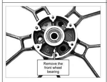
[7] If the front wheel bearing is seriously worn and damaged, the front wheel bearing shall be knocked out gently with the axle bearing removal tool and replaced with a new bearing.
