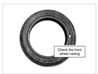
[9] Check the wear condition of the front wheel tread. The repair limit value of the tread wear of the front wheel tread is 2.00mm. During the use of motorcycle, if the front tire pressure is insufficient, first check the inner tube valve core for air leakage, and then check the inner tube for air leakage.
