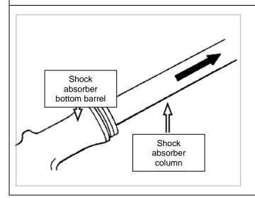
[5] Remove the front shock absorber column and the front shock absorber bottom cylinder, check whether the front shock absorber column and the front shock absorber bottom cylinder are worn, and replace the front shock absorber column and the front shock absorber bottom cylinder when they are worn.
