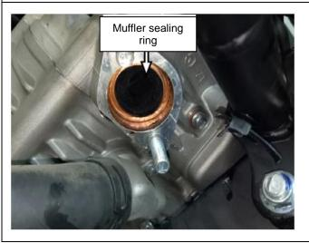
[3] Remove the muffler sealing gasket and check whether the muffler sealing gasket is damaged. When the muffler sealing gasket is damaged, replace it with a new one.
