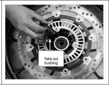
[5] Take out the front axle oil seal and check the wear condition of the front wheel oil seal cutting edge. If the front wheel oil seal cutting edge is seriously worn, it should be replaced.
