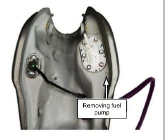
[6] Remove 6 M412 fixing bolts of fuel pump with Allen wrench tool.
