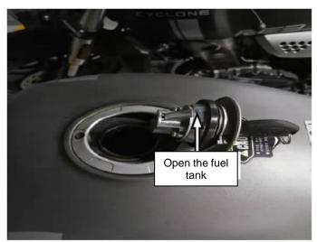
[3] Check the fuel tank for oil leakage. If oil leakage occurs in the fuel tank, the fuel tank must be repaired or replaced.
