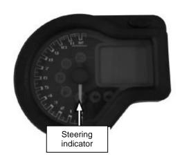
[4] Check whether the indicator bulb of the instrument is burnt out. When the indicator bulb of the instrument is burnt out, replace the indicator bulb of the instrument.
