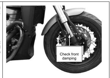
[2] Remove the front shock absorber fixing bolt and remove the front shock absorber.
