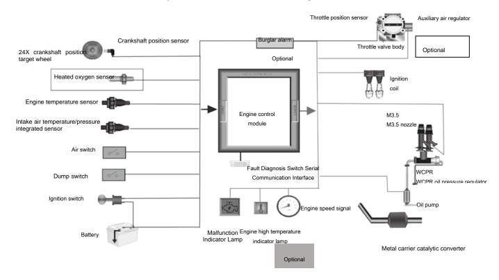
Structural schematic diagram of EFI system
