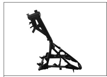
The frame is a plate welded frame with a high strength, good rigidity and strong applicability. It mainly consists of the front section of the frame, the frame tail frame and the engine bracket.
