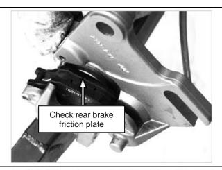
[12] Remove the friction plate of the rear brake and check the wear condition of the friction plate. Its maintenance limit is 2.0 mm.
