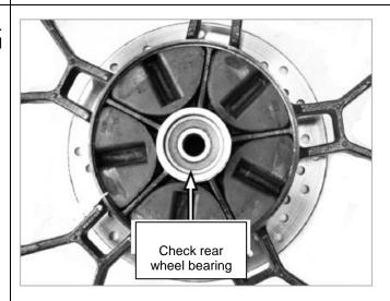
[13] Check whether the front and rear aluminum wheels are deformed, timely correct the front and rear aluminum wheels or replace the aluminum wheels. Check whether the tread pattern of the rear wheel is worn. When the tread pattern of the rear wheel is worn beyond the maintenance limit of 2mm, the rear wheel tread needs to be replaced.
