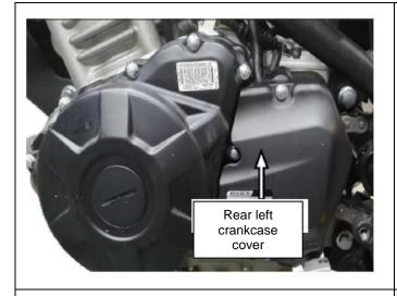
[2] Remove the fixing bolts of the left rear case cover of the left crankcase body and the left rear case cover of the left curved shaft case body.
