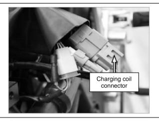
[3] Remove the magneto charging coil socket, and use a multimeter to measure whether the magneto charging coil is short-circuited. When the magneto charging coil is short-circuited, replace the magneto charging coil.
