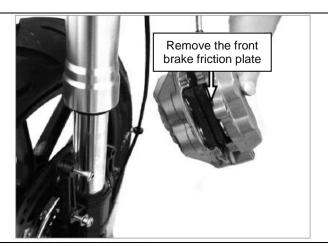
[3] Remove the disc brake friction plate and check the working condition of the brake caliper piston. If the brake caliper piston cannot operate normally, the hydraulic brake must be repaired or replaced.
