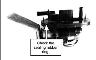
[8] Check whether the sealing rubber ring of the fuel pump is aged or cracked, whether there is oil immersion, and if so, replace the sealing rubber ring of the fuel pump.
