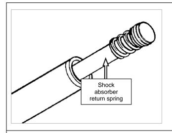
[6] Take out the return spring of the shock absorber column and check whether the elasticity of the return spring is worn or deformed, and replace it when the return spring is deformed.
