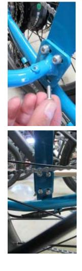
Install the running board frame rear mounting bolts. Tighten
