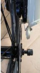
Make sure the axle is seated all the way up in the fork dropouts. Using the 15mm wrench, tighten down the axle nuts.
