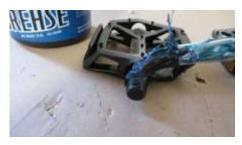
Using the 15mm wrench, install the pedals as shown.
