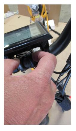
Install all four handlebar clamp Allen bolts, and lightly tighten them. Make sure the bars are centered. Rotate the handlebars to your preferred angle and finish torque the allen bolts.
