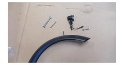
Run the fender mounting bolt through the headlight, fender tab, and fork crown as shown.
