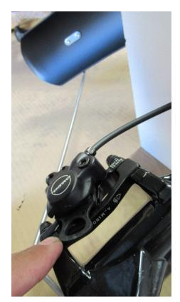
Remove the plastic spacer from the front disc brake caliper.
