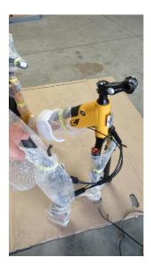
Using the 4mm hex key, remove the handlebar clamp from the stem.
