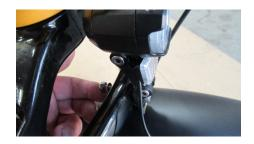
Using the 5mm hex key and 10mm wrench, snug up the main fender mounting bolt.
