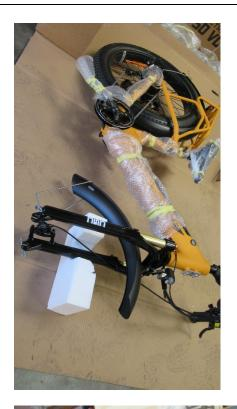
Using the 4mm hex key and 8mm wrench, install the fender stays, left and right, as shown.
