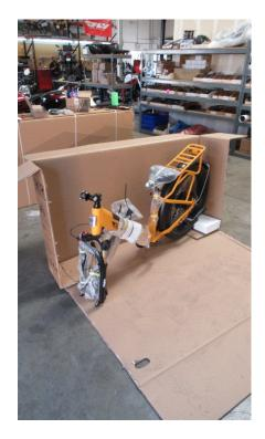
Pro Tip: While the bike will free-stand, put down the kickstand, and use the styrofoam to help stabilize it.
