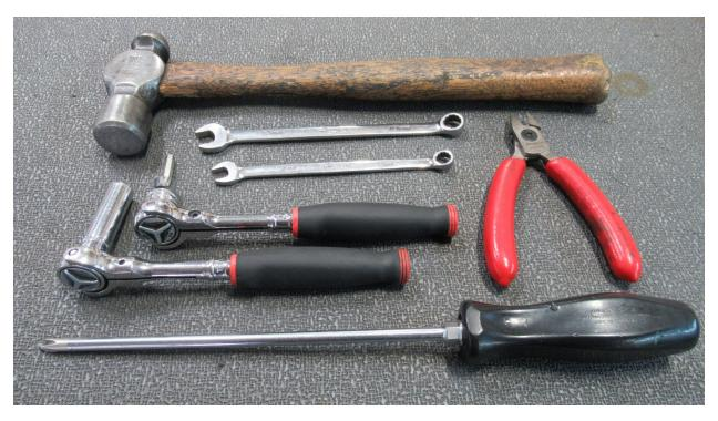
Tools needed: Phillips screwdriver, side cutters, 10mm socket with ratchet, 5mm Allen, 8 &10mm wrench, hammer
