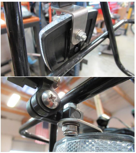
22. On the front of the basket, assemble the front reflector and headlight with the stock 8mm washer and nut.
