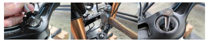
3. Using a star nut driver and hammer, install the star nut in the steerer tube. If a star nut driver is not available, fully insert the long 6x45mm bolt (supplied) and carefully drive the star nut 3/4" inch into the steerer tube. Removing the forks and bringing them to your local bike shop is also an option
