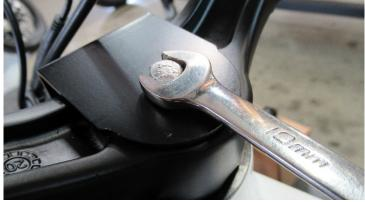
4. Install the lower basket bracket with the long 6x45mm bolt and washer. Leave loose enough to adjust
