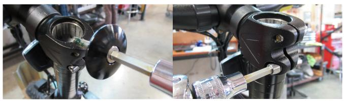
7. Using a 5mm Allen, remove the top cap and loosen the (2) stem pinch bolts
