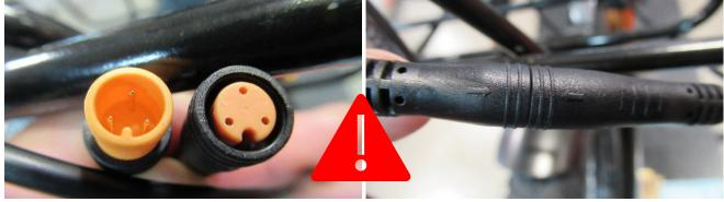
23. Connect headlight connector. Caution, it only goes in one way. Line up internal tabs or arrows on the connector
