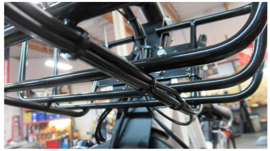
24. Route the USB and headlight wires underneath basket to protect the wires
