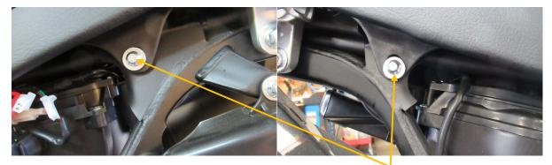
With a 8mm wrench or socket, remove the left and right seat bolts and washers
