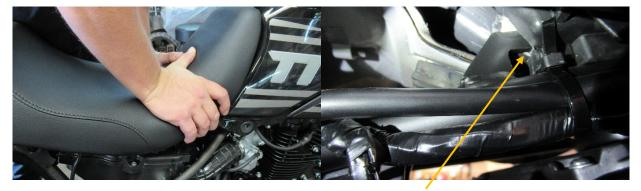
Push firmly down and forward to engage seat pan onto the hooks on the frame
