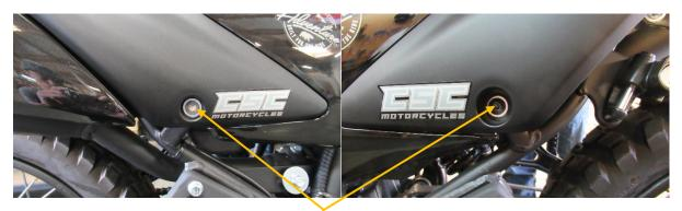
With a 5mm Allen, remove the silver button head Allen bolts on the right and left side panels
