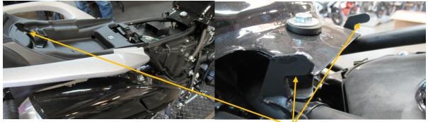
Push seat rearwards to unlatch seat pan from the hooks on the frame
