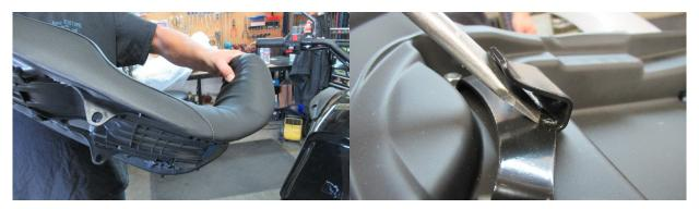
To ease installation of the lowered seat, create additional clearance by pulling back on the nose of the seat and prying up on the rear seat hook
