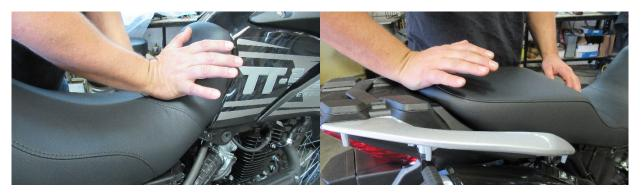
With the heal of your palm, firm shoves forward will help fully engage the seat. Verify the rear hook is engaged to the seat pan.
