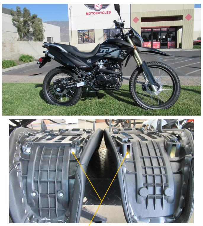
The CSC lowered seat by Seat Concepts lowers your riding position by 3 inches. To achieve this, a different seat pan is used which have smaller hook cutouts. Due to shorter profile and the flexible nature of the seat, additional steps and techniques need to be used for installation. Tools needed can all be found in your tool kit.
