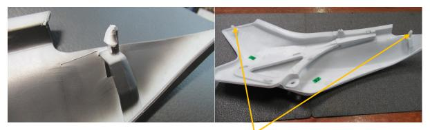
Pull the top corners of the side panels out to release the "mushroom pins" from the rubber gromets
