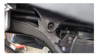
Align the seat so the hole in the pan lines up with the threaded hole in the frame
