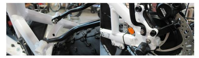
With an 8mm wrench, loosely install the rack bolts with washers until all (4) bolts are installed. Shorter 5 x 10mm bolts are used on the top. Evenly tighten and readjust rack if necessary. Replace zip ties
