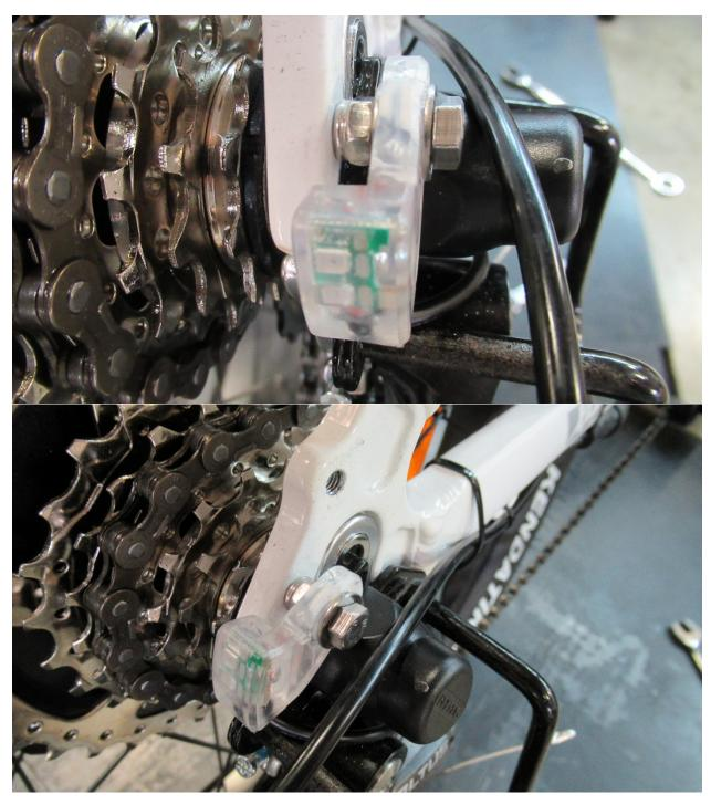
It may be necessary to gently pull a little slack from the wire for the light to reach the lower mount. Cut zip ties if necessary. Install right rear taillight assembly into lower accessory threaded mount. To prevent damaging the light, not to over tighten
