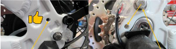
On the 2021 XP models, because to the taillights, rear racks are mounted to the **upper** accessory threaded hole on the rear wheel dropout.
