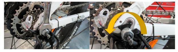
Additional clearance will be needed from the derailleur guard to the threaded hole to install the light assembly. With a 18mm wrench, loosen the axle nut and reposition the derailleur guard by turning it counter-clockwise until it stops. Firmly retighten axle nut.
